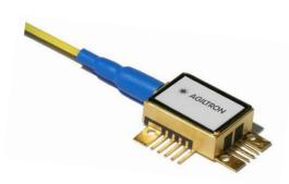
The FORX Linear Photoreceiver is designed for high-speed and high sensitivity analog and digital applications, featuring a surface-coupled coplanar waveguide APD photodiode and a linear transimpedance amplifier within a hermetically sealed package. Its high conversion gain and low input-referred noise ensure exceptional linearity and precision.
